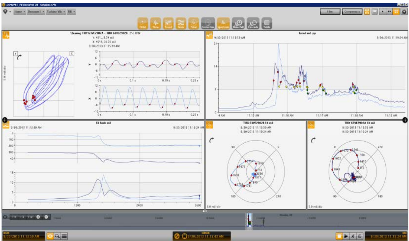
Figure 6: Typical screen from condition monitoring software using data provided via the Machinery Engineering Information Interface. It augments the information available via the Operator Information Interface by providing detailed waveform and other high-speed, high-bandwidth data needed for the specialized plot types used by machinery and vibration analysts.
