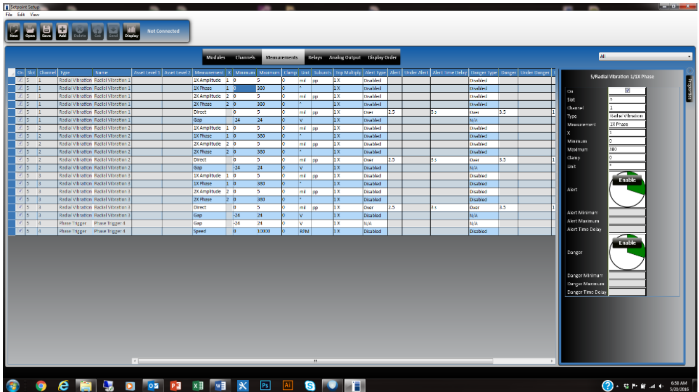
Figure 7: Typical screen from configuration utility. It allows every aspect of the protection system to be changed. As such, access to this port must be carefully controlled and represents one of the most potentially vulnerable points in the system’s connection to the outside world.
