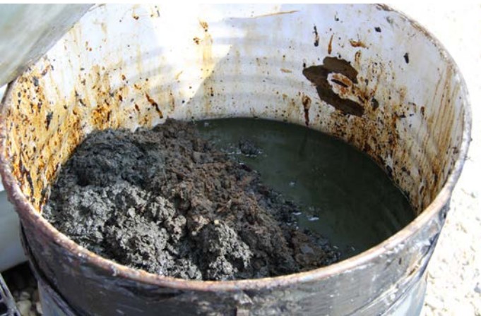
Left: Sand, Wax and Solids Removed in Crude Oil Treater. Below: Clamp-on Ultrasonic Transducer Monitoring Crude Oil Flow in 3" Steel Pipe
